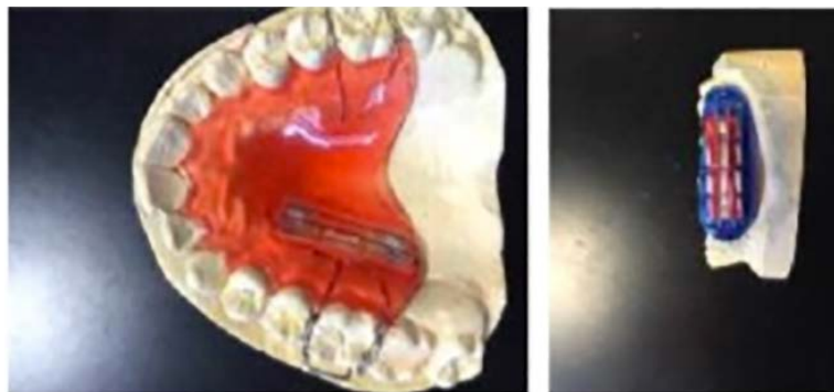
Figure 15. Human enamel specimens mounted into appliances worn for human in situ erosion prevention studies.
